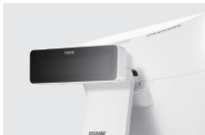
Customer Display • VFD (2 Line x 20 Characters)
