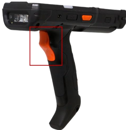
Figure 72 Gun handle - Scan button
