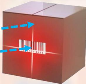
The TC8XXX senses that a box has been waved in front of it, using its proximity sensor, and activates the scan engine to decode the barcode.
